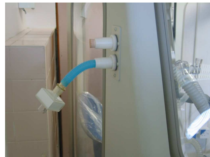
Outlet HEPA filter
