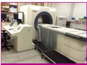
Fig 1: JC high-intensity focused ultrasound system (Personal collection)
