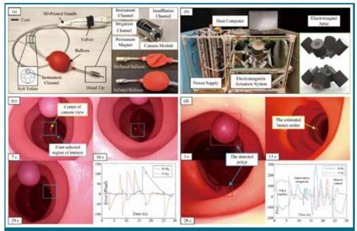
Fig. 3. Electromagnetically actuated soft-tethered (EAST) colonoscope system developed by Li et al. in CUHK. (a) Prototype of the soft-tethered colonoscope with an inflatable balloon and a magnetic tip. (b) Small-scale prototype of the electromagnetic actuation system for proof-of-concept. (c) Automatic region-of-interest tracking based on visual servo control. (d) AI-based autonomous colon navigation with automatic polyp detection. (Adapted from reference<sup>27-29</sup>)
