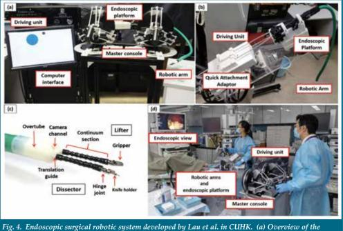
endoscopic surgical robotic system. (b) Overview of the driving unit. (c) Overview of the robot arms. (d) Experimental setup of the in-vivo experiment. (Adapted from reference<sup>34-37</sup>)
