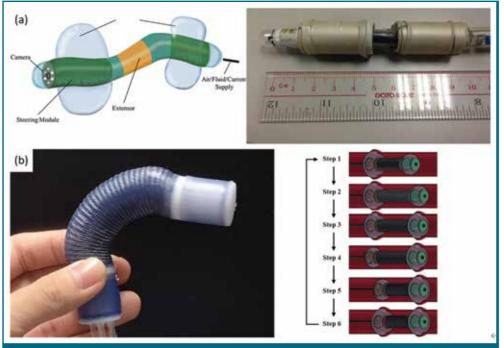
Fig. 2. Earthworm-inspired endoscopes developed by Poon et al. and Zhang et al. in CUHK. (Adapted from reference<sup>21-23</sup>)
